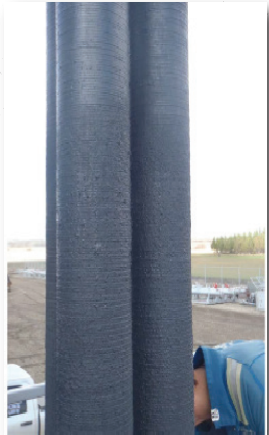
Stacked Barrier Plates inside the MegaPOL
