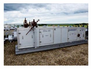
MAWP: 1,480 psi [10,200 kPa] ANSI: 600 MDMT: -50°F [-44°C] DESIGNATED SERVICE: Sour WEIGHT (EMPTY): 11,500 lb (4,985 kg) LENGTH: 26.6ft (7.3 m) LIQUID VOLUME: 8.35bbl (1,129 L) SAND CAPACITY: 4,923 lb (1,905 kg) FITTING CONFIGURATION: 3" flanged
