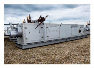
MAWP: 5,450 psi [37,577 kPa] ANSI: 2500 MDMT: -50°F [-44°C] DESIGNATED SERVICE: Sour WEIGHT (EMPTY): 9,070 kg LENGTH: 7.6 m LIQUID VOLUME: 443 L SAND CAPACITY: 741 kg FITTING CONFIGURATION: 3" flanged
